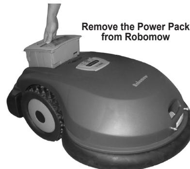
Remove the Power Pack from Robomow
