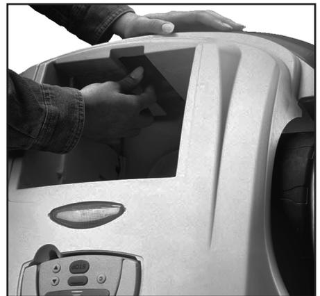
To adjust ground clearance, pull out on tab as shown and slide tab up or down.
