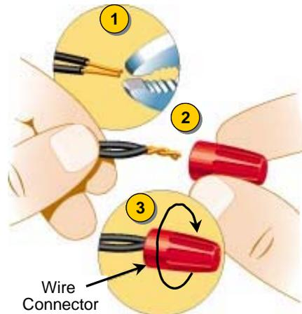
1. Strip 1cm (0.5 inch) of each wire ends together and twist the stripped ends together using pliers.
