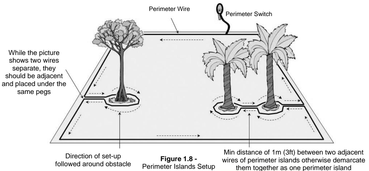
**Caution!** Setting the Perimeter Wire counter-clockwise around the obstacle will cause Robomow to drive into the island".
