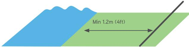
Alternatively, place a physical barrier close to the water.
