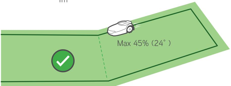
Exclude any slope greater than 20% that are on the edge of your lawn to prevent the mower from slipping outside your lawn (especially in wet conditions)
