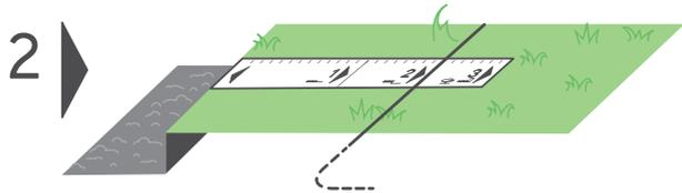
When the edge is a wall (more than 2 cm/ 1" above the ground level), use the 3rd distance of the RoboRuler.
