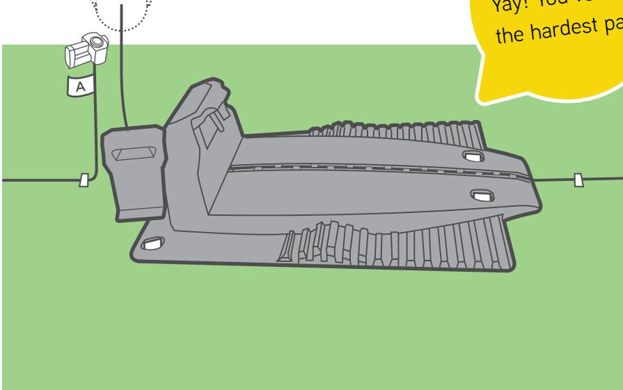
Peg the wire to the ground. Twist and wrap the wires so they could fit nicely in Base Station compartment. Connect the wire end marked with 'A' to the connector marked with A on the back of the Base Station. Connect the other end to the other connector. Tuck the wire in and close the door.
