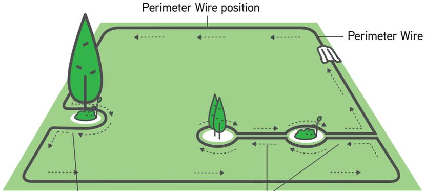
If the distance between an island and the perimeter wire is lower than 1.2m (4 ft), make the obstacle part of lawn's edge.
