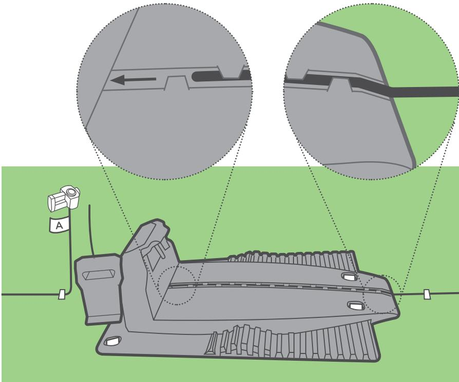
Install the connector to the tip of the wire as described in the drawings. Cut the wire end, close to the connector.
