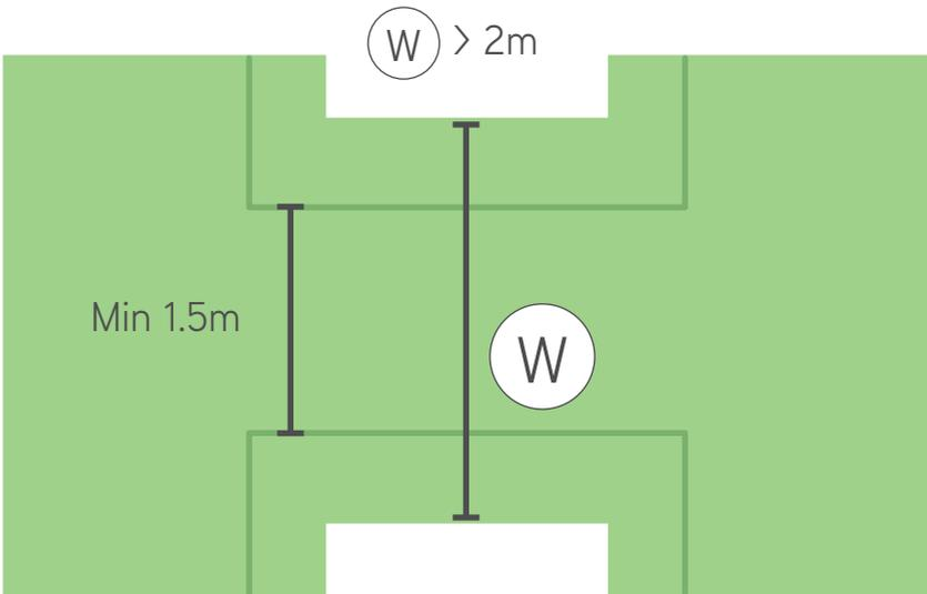
When a narrow pass is between 1-2m (3-6ft), the wires should be installed in the middle of the path with RoboRuler distance 1 between them to allow the mower to be able to follow the wires in and out of the sub zone. On the entrance to the path from both directions, you should break the corner to 45 degrees so the mower will turn accurately in and out the narrow pass.
