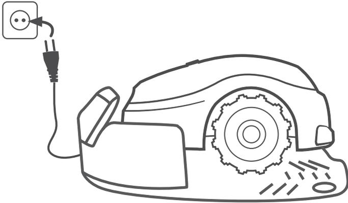
**i** Take the power cord out of the mowing area (to prevent the mower from damaging it) and secure the cord firmly to the ground (so that it does not become a tripping hazard).
