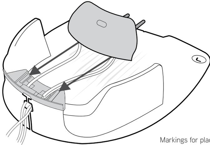
Markings for placing the Base Station Head
