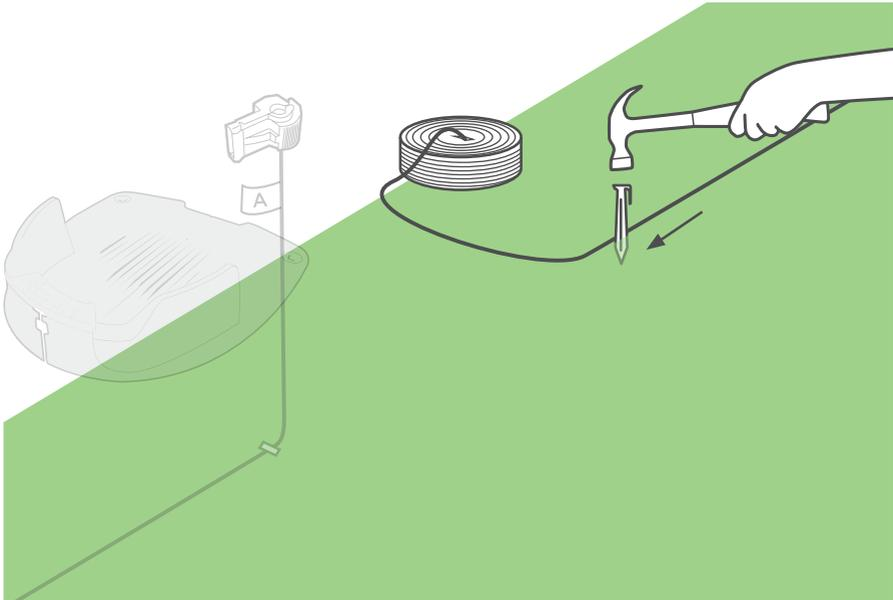
Make both wires end the same length. Use a cutter to cut off the remaining wire. Do not leave or create wire wraps
