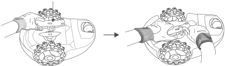
4. Use the provided Allen tool (comes with a replacing blade) to unscrew the screws while holding the blade with the RoboTool.
