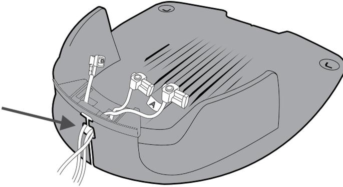
2. Connect the wire tail marked A to the A terminal and the other tail to the B terminal of the Base Station head.
