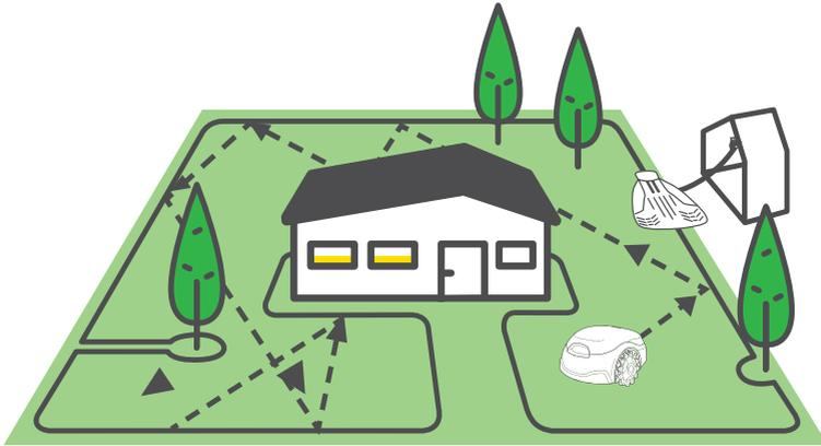
At the end of each mowing ride, your mower will follow the Perimeter Wire and automatically return to the Base Station for charging.
