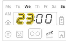
Set the time, at which the Inactive Hours start and press **OK**.
