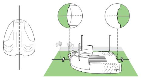
• Fix the base to the ground with the 4 supplied metal stakes
