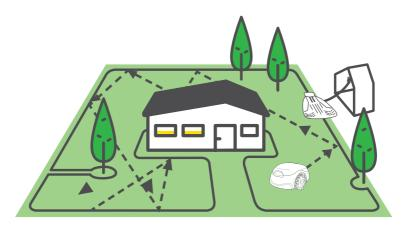
At the end of each mowing ride, your mower will follow the Perimeter Wire and automatically return to the Base Station for charging.
