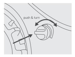
To set the mowing height, push and turn the mowing height adjustment knob to the desired direction:
