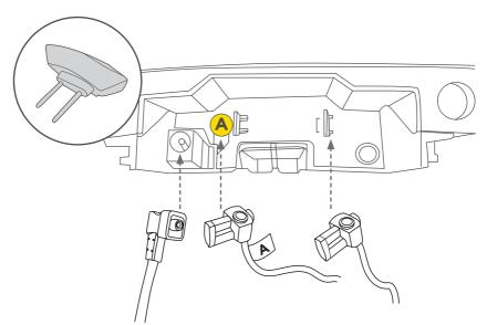
4. Place the head on the Base Station head adapter and align it with the markings as shown in the picture below.
